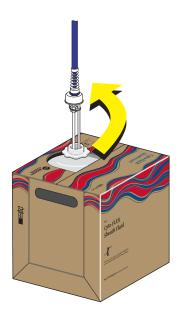
**4** Inspect the pickup tube assembly and replace it if necessary.
